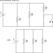
So, equivalent resistor =  $\frac{R}{3} = \frac{9}{3}\Omega = 3\Omega$
